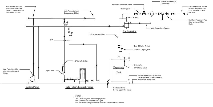
Detail : Heating Water Expansion Tank & Side Filter / Chemical Feed System (w/o Glycol)
