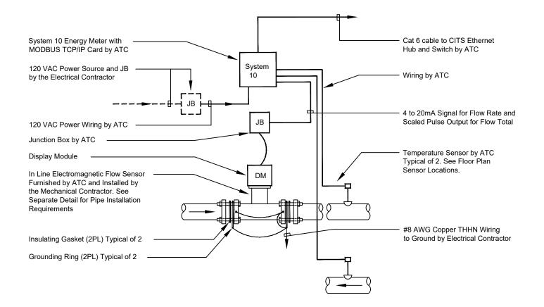
Condenser Water System - Non Metallic Pipe Installation - Ethernet Application Detail:Installation - In Line Electromagnetic BAS Energy Meter
