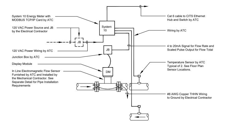
HVAC Hydronic Systems - Metallic Pipe Installation - Ethernet Application Detail:Installation - In Line Electromagnetic BAS Energy Meter
