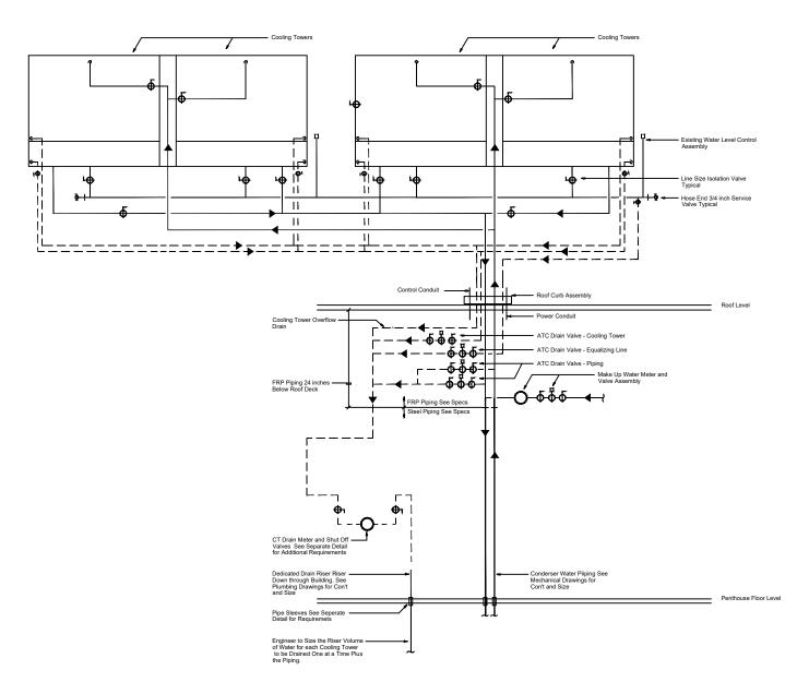
Detail - CT Automatic Drain and Fill
