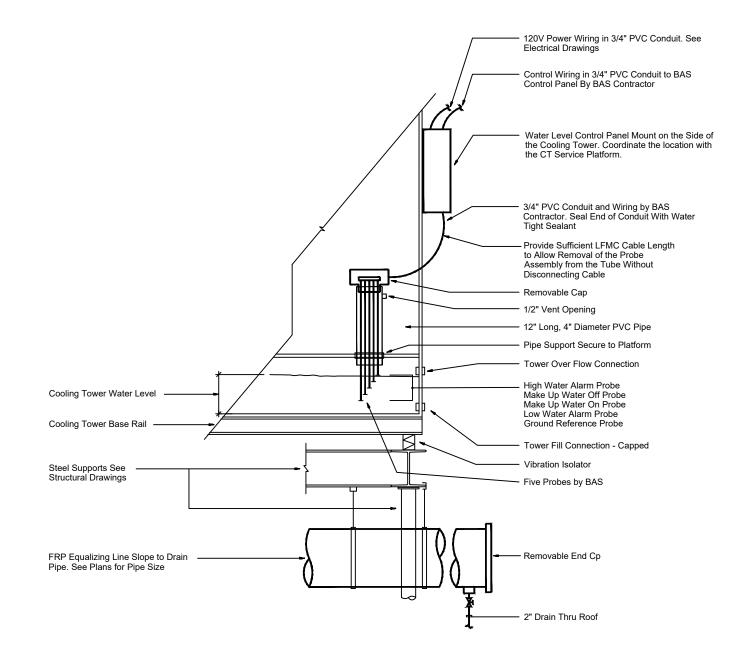
Detail - Cooling Tower Internal Water Level Controller
