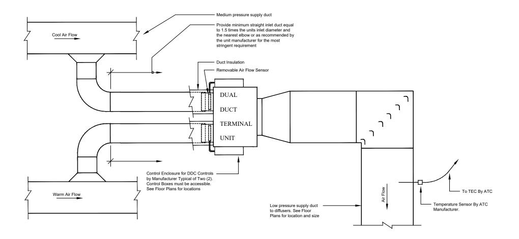
Detail : Dual Duct Terminal Unit - Ductwork
