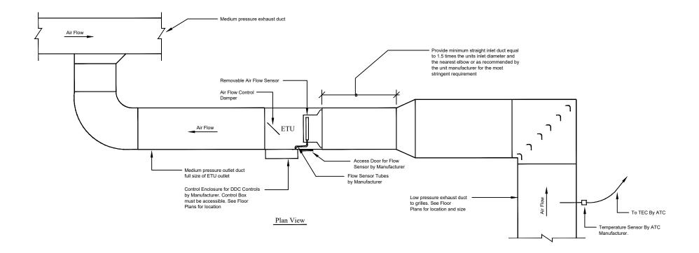
Detail: Square Exhaust Terminal Unit - Ductwork
