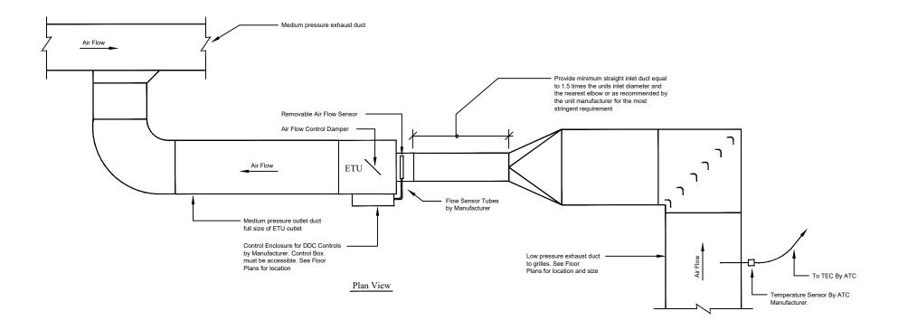
Detail: Square Exhaust Terminal Unit - Ductwork
