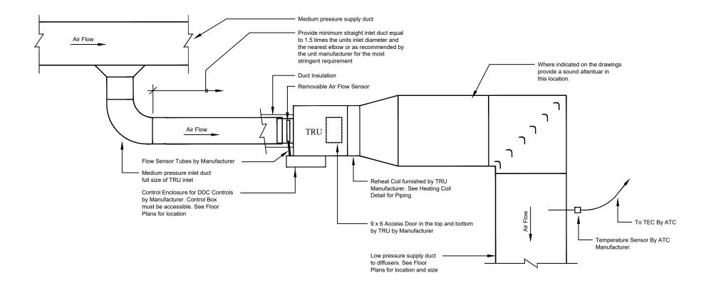
Detail: Terminal Reheat Unit - Ductwork
