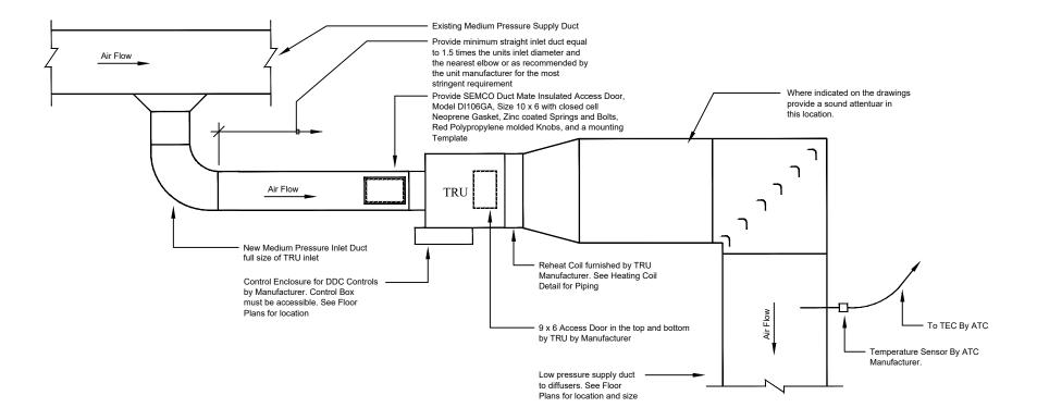
Detail: Terminal Reheat Unit - Ductwork w/ Access Door
