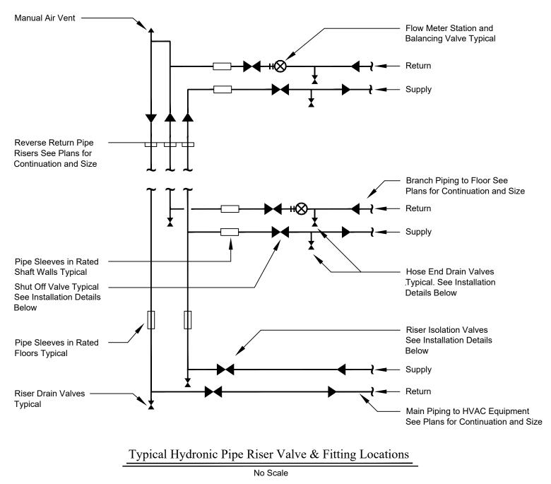
Contractor Note: Reverse Return Piping Systems are Typical for Chilled Water, Process Cooling Water, Heating Water, and Energy Recovery Piping Systems.
