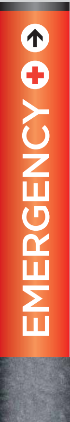
Free-standing Emergency Directional (FS EM sign) Emergency signs will be upgraded with a granite base, DOT hospital cross pictogram and a distinctive lozenge profile. Though internal illumination might be the ideal way to increase visibility, a bright red porcelain enamel background will also be distinctive.
