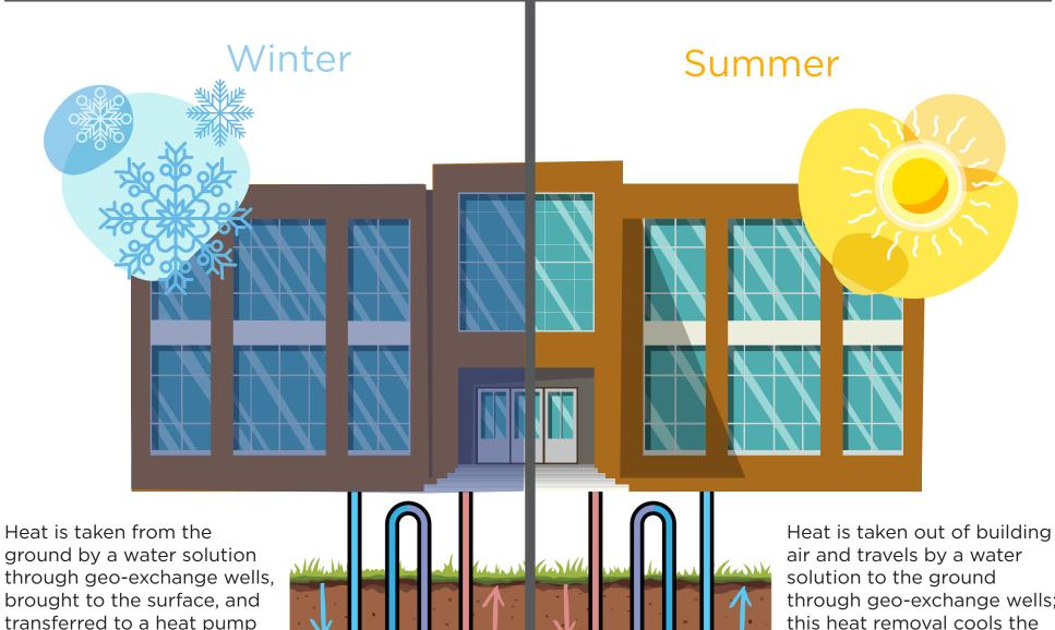
ground by a water solution through geo-exchange wells, brought to the surface, and transferred to a heat pump that warms spaces in the building.
