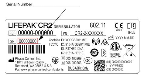
6. Check the date of manufacture on the battery label, printed in YYYY-MM-DD format. The battery must be installed within 1 year of this date to attain a 4-year service life. For detailed information about battery service life and maintenance, see Maintaining the Battery (on page 81).
