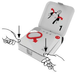
5 Press down on the front corners of the electrode tray until it clicks into place. IMPORTANT! When you insert the new tray, be careful to press only on the corners of the tray where the foil is supported. Pressing on the center of the tray may damage the seal and cause the electrodes to dry out.
