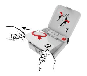
2 Pull the electrode tray up and out of the defibrillator.
