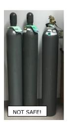
When working with compressed gas cylinders, lab members should be adequately trained on the proper use, handling, storage and disposal. Although the actual container may look harmless, keep in mind that compressed gas cylinders pose mechanical, physical, inhalation, and/or other health hazards if used carelessly.
